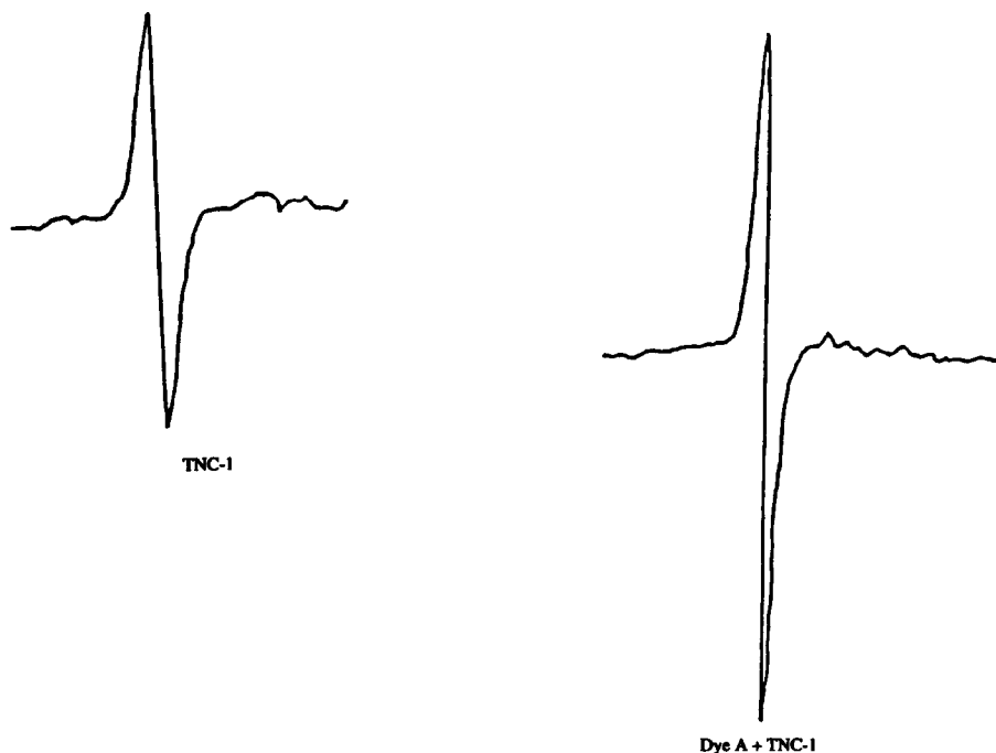
Fig. 3. Light-induced ESR signal of emulsion with TNC-1 and dye A + TNC-1.
